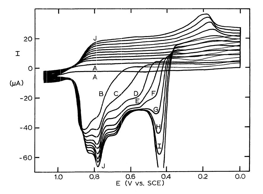
Figure II-10. Dependence of limiting current on rotation speed of Au disk during negative scan of potential for Hg(II) in 2.0  $\underline{M}$  HNO<sub>3</sub>
