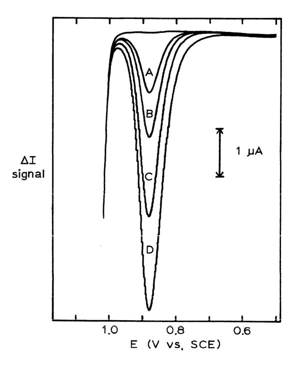
Figure III-11. Dependence of the DPASV peak-area on  $V_{f,dep}$ , at constant  $V_s$
