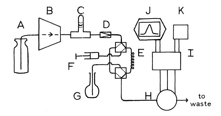
a bubble of air (~0.25 mL) in series with the adjustable needle valve (D), described above, for generation of back pressure. The inverted T-tube was marked in such a way that the position of the meniscus gave an approximate indication of the back pressure supplied by the needle valve, e.g., 3,10,15,20 psi, etc. The sample loop for these experiments had a volume of 0.145 mL.
