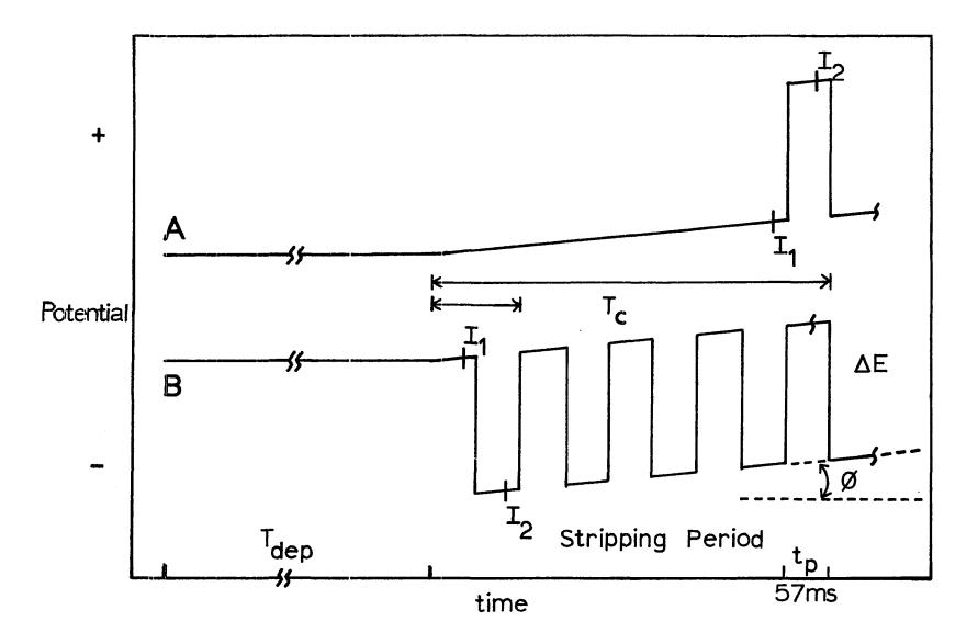
The current,  $I_1$ , measured just prior to application of the pulse is subtracted from  $I_2$ , the current measured just prior to the conclusion of the pulse. The difference is amplified and passed to the recorder as  $\Delta I$  according to Equation III-1.
