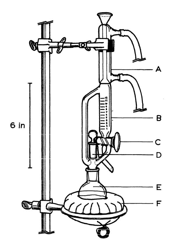
distillation arm of the apparatus was wrapped in asbestos. The reaction vessel was a 50-mL round-bottom pyrex flask from Ace Glass Co., Louisville, KT.
