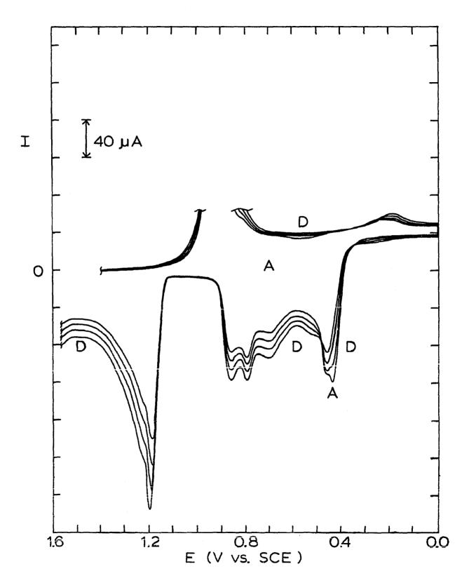
Figure II-14. Comparison of currents obtained at Au disk for a surface-controlled process and for UPD of Hg(II) in 2.0  $\underline{M}$  HNO<sub>3</sub> as function of rate of potential scan
