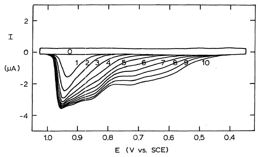
Figure II-17. Charge passed during stripping of UPD Hg from tubular Au electrode in 2.0  $\underline{M}$  HNO<sub>3</sub>
