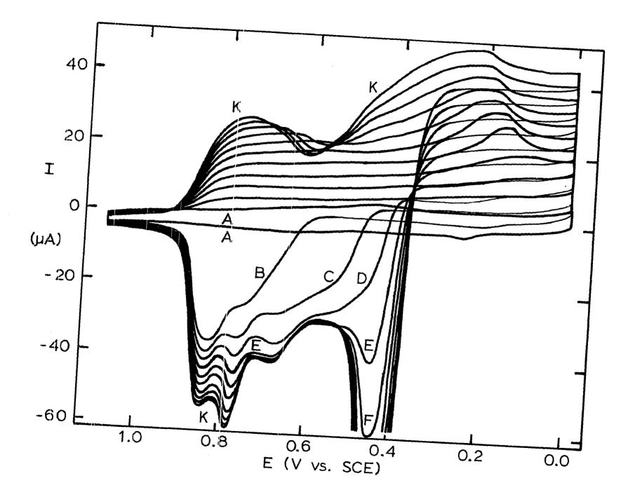
Figure II-8. Limiting current produced at Au disk during negative scan of potential for various concentrations of Hg(II) in 2.0  $\underline{M}$  HNO<sub>3</sub>
