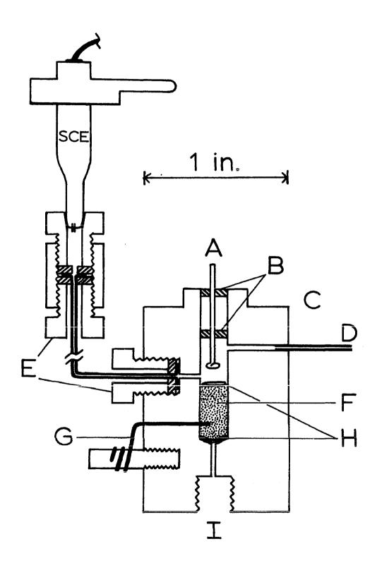
$\sim$ 1.0 cm. Electrical contact to the chips was made by a 20-gauge Au wire (G) protruding through the detector body into the chips.
