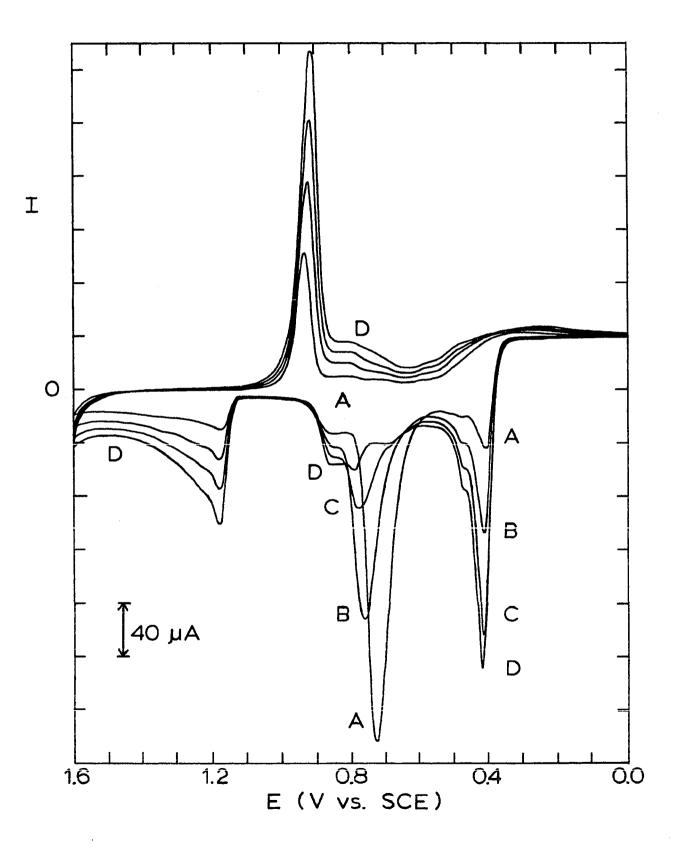
Figure II-12. Effect of rate of potential scan of Au disk for Hg(II) in 2.0  $\underline{M}$  HNO<sub>3</sub>
