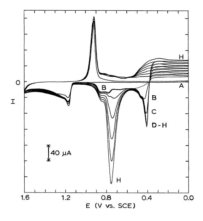
Figure II-6. Dependence of limiting current on rotation speed of Au disk during negative scan of potential for Hg(II) in 2.0  $\underline{M}$  HNO<sub>3</sub>
